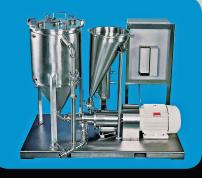
A portable, self-contained powder injection system can serve multiple process lines instead of just one.
