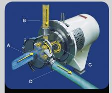
In the SLIM (Solid/Liquid Injection Manifold) powder-injection system, a liquid stream (A) enters the highspeed rotor. Drawn into the mixer by a powerful vacuum, the powder (B) is injected through the ported rotor (C) directly into the high-shear zone, where it is subjected to intense shear. With particles instantly dispersed, the resulting product is ejected from the mixer (D).
