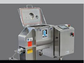
This laboratory ribbon blender is equipped with a PLC-driven control system with a touch screen interface. As product development proceeds, every process variable is controlled, and each batch is documented.
