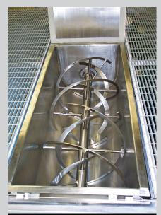
A ribbon blender engineered for sanitary applications includes highgrade stainless steel construction, a sanitary finish, close tolerances, and design details that eliminate corners and crevices where batch material might collect. to protect against phase failure and under-voltage.
