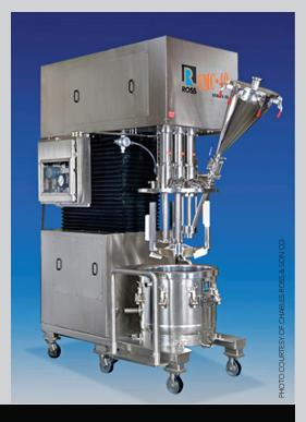
A fully enclosed multi-shaft mixer provides increased control over critical process parameters such as temperature and pressure. Because the agitators are independently driven, the unit can operate with various combinations of high-shear and low-shear agitators in process. Numerous operations can be accomplished in a single unit—eliminating the time, expense, and risk of contamination associated with transfers between several single-agitator mixers.
